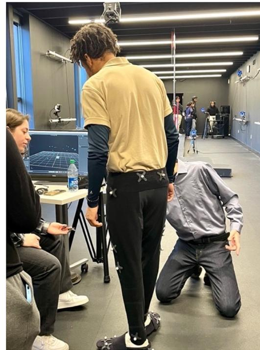
Cameras interact with the markers and the information is encoded and transmitted to a computer.
